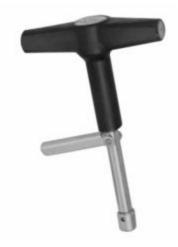
Measures torque when turned in a clockwise direction & ratchets when turned counterclockwise When the brand screw is tightened to the correct torque, the wrench ratchets so the handle will continue to turn but the drive socket will not Retractable reversing lever Chrome vanadium socket
