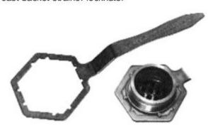
Fits 3-1/2" plastic locknuts Fits 3-3/8" die cast basket strainer locknuts Fits brass locknuts on brass shower stall drains Stamped steel 13" overall length Offset handle for close quarter work Cushion grip
