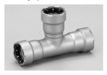
Viega MegaPressG fittings are provided with a factory installed HNBR sealing element, a 304 stainless steel separator ring and a 420 stainless steel grip ring and are CSA LC4 approved for fuel oil and fuel gas installations.
