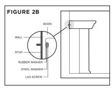
7. Tighten hex nut (stud application) or toggle bolt (wall application) until pedestal basin is snug against the wall.
