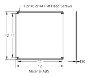
**Installation Note:** Panel shall be attached with construction adhesive or with screws directly to the front of finish wall. Panels shall have countersunk holes for flush screw finish and will receive #6 or #4 flat head screws.
