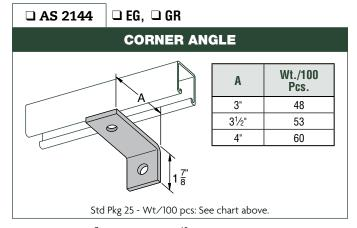
Page notes unless otherwise specified: 1/4" thick, 15/8" wide, holes 9/16" diameter, spaced 17/8" on center and 13/16" from end.
