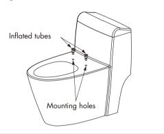
3. Place the Fixed Card on the toilet bowl where the mounting holes are. Make sure that the wash / dry gates are close to the rim and pointed down
