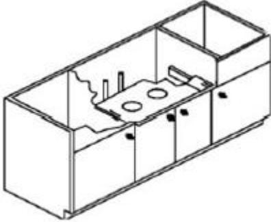
Apron sinks require a base cabinet with an opening in the front of the cabinet. In addition, unlike a standard undermount or top mount sink which may be supported by a countertop, this sink should be supported independently by the cabinet. The support should be sufficient for the weight of a completely filled sink plus any attachments such as garbage disposals and an additional safety factor. A licensed contractor should be able to design adequate support.
