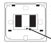
Gas: For systems that control the fan during a call for heat, put the fan operation switch to the GAS position. Electric: For systems that do not control the fan during a call for heat, put the fan operation switch to he ELECTRIC position.
