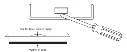
Gently slide a screwdriver into the bottom edge of the badge. Gently turn the screwdriver counter clockwise. The badge is held on by a magnet in the well of the battery door. The badge should pry off easily. DO NOT USE FORCE.
