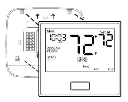
Align the 4 tabs on the subbase with corresponding slots on the back of the thermostat, then push gently until the thermostat snaps in place.
